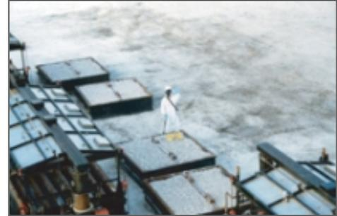
this contract, Parsons treated the excavated 15,000 tons of soil contaminated with Agent Orange and 15,000 tons of soil contaminated with PCBs and/or heavy oils. The thermal treatment included screening of all soil and briquetting the fine-particle soil prior to treatment. This contract also required that Parsons put into operation an extensive air emission treatment system along with a wastewater treatment plant that was also required under the thermal treatment contract.
